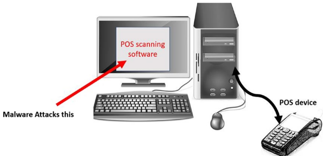
Figure 15-3. The POS device and the PS software setup which is the target of malware
