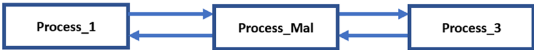
Figure 11-29. A list of processes, including a malware process represented in the kernel
